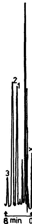
Fig. 1. Chromatogram of a 50- \mu l extract of liquid plasma from a patient following oral administration of a dapsone/chlorproguanil combination. Peaks: X = Injection; 1 = I.S. (1 \mu g); 2 = DDS (1.22 \mu g/ml); 3 = MADDS (0.25 \mu g/ml). Comparable chromatograms were obtained from filter paper-absorbed samples.
